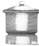
No. 683 - Fruehling & Schultz Desiccating Jar, Ground Cover with Knob 1909 Number: No. 42 - Desiccating Jar Hand made, heavy weight Inside Dia x Inside Ht sizes: #683/1 - 8"x8" #683/2 - 10"x9 1/4"
