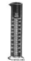
No. 657 - Graduated Cylinder with lip & foot, Metric Scale, Reading Up and Down Available sizes - Capacity - Dia x Ht: 5cc - ¾"x3¼" 10cc - ½"x3¾" 15cc 25cc - ¾"x5½" 50cc - 1 5/16"x6¾" 100cc - 1 1/8"x9¼" 125cc 150cc 200cc - 1 1/8"x11 250cc - 1 1/2"x11 3/4" 300cc 500cc - 1 15/16"x13 3/4" 1000cc - 2 5/16"x17 1/2" 1500cc 2000cc Available with optional Carmen Lines & Figures, Acid Etched
